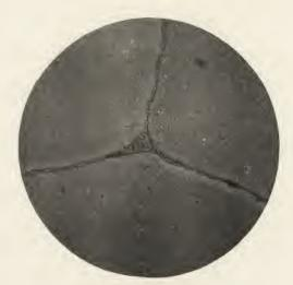
Fig. 17 Type of Class 2. Iron containing 1.8 per cent. P. Magnified 350 diameters.
